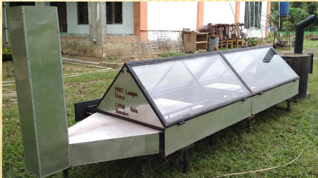
The fabricated HGSD attached with biomass burner
