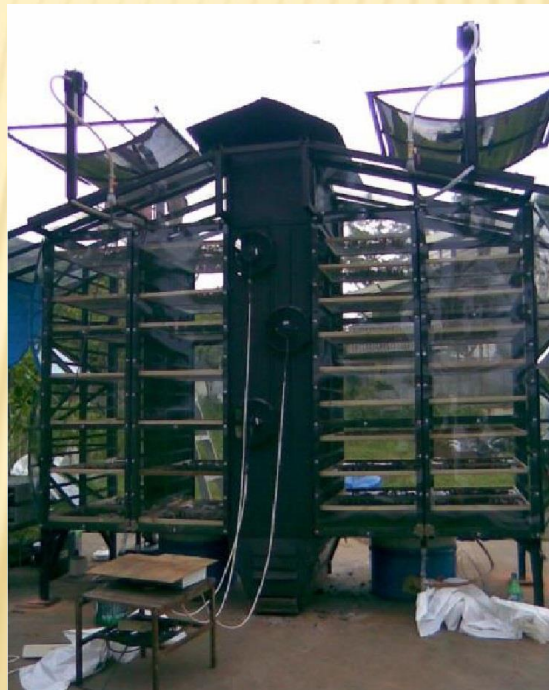
Rack-type greenhouse attached with biomass burner
