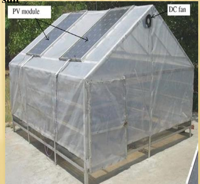
Setup of greenhouse dryer operating under active mode
