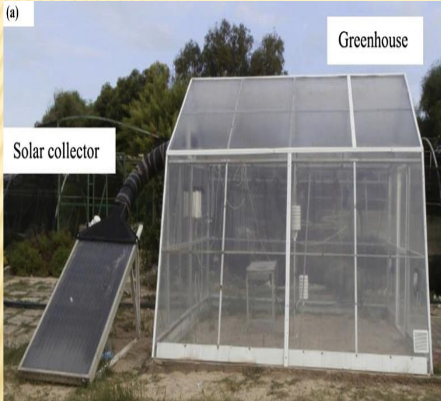
(a) Direct type dryer attached with flat plate collector (b) Dryer with the opaque north wall
