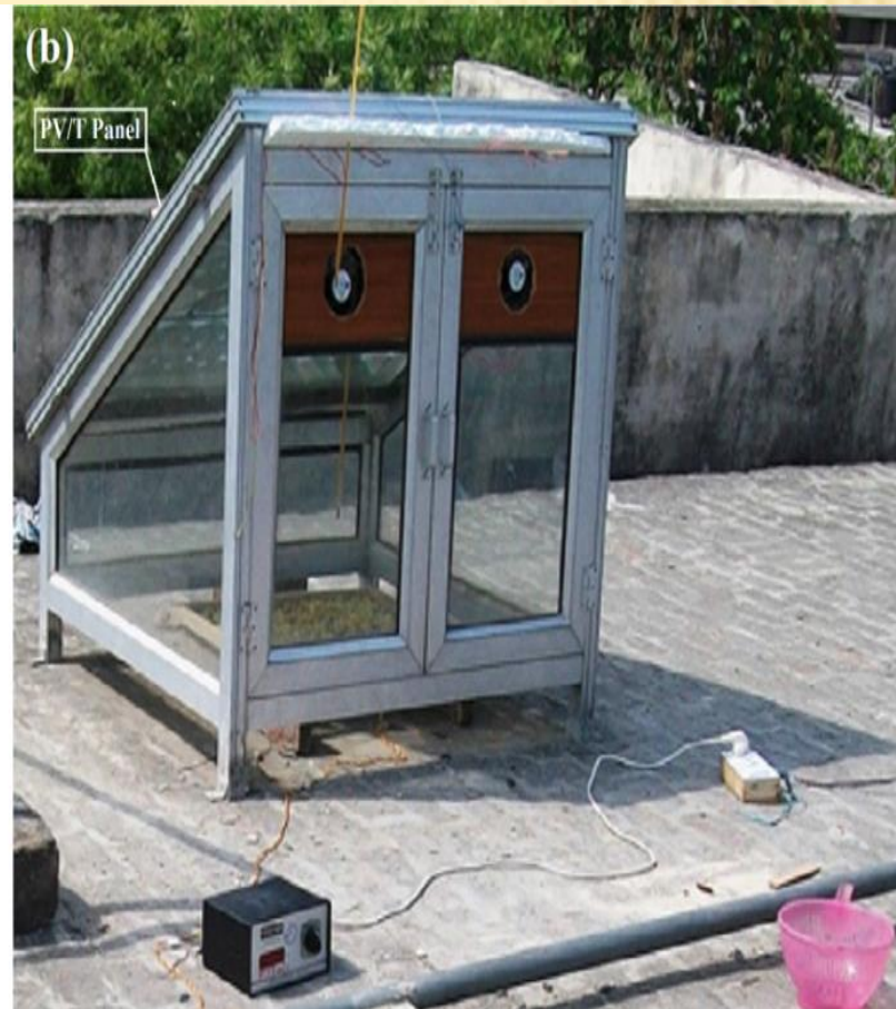
a) Reverse absorber natural convective solar dryer (b) Dryer with PV/T Panel
