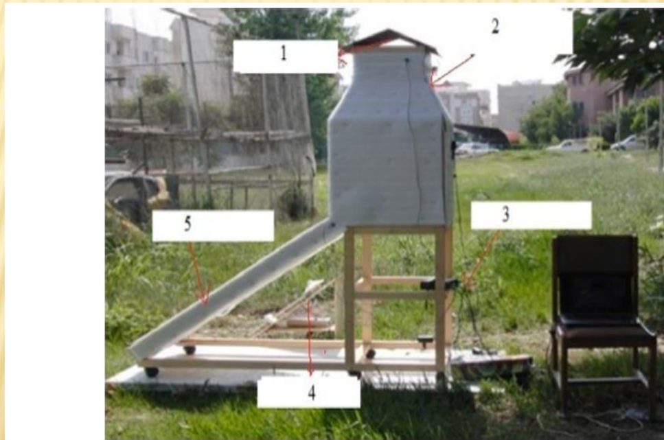
1. Hot air outlet 2. Dryer cabinet 3. Thermocouples 4. Pyranometer 5. Solar air heater
