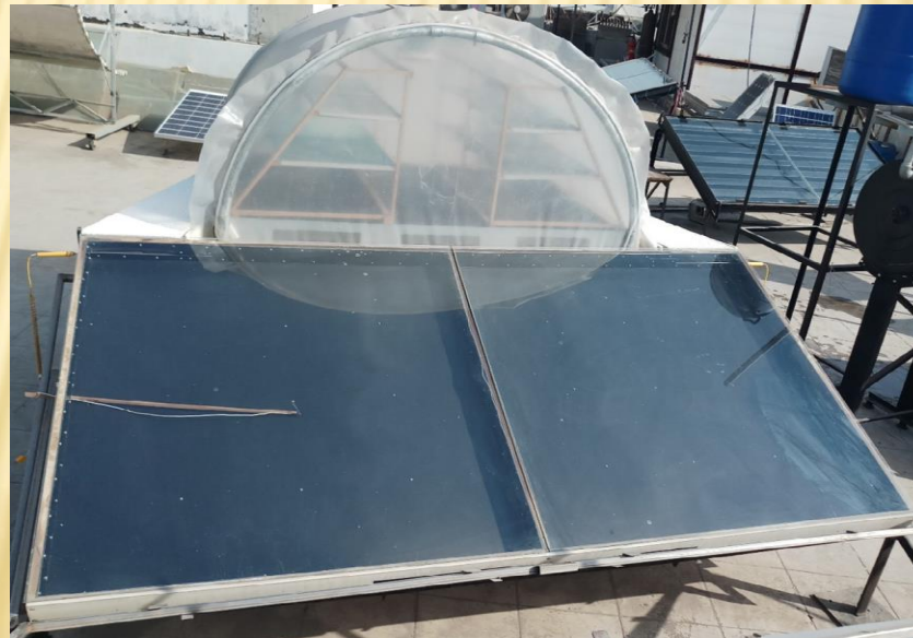
Rack-type HGSD attached with flat-plate collector
