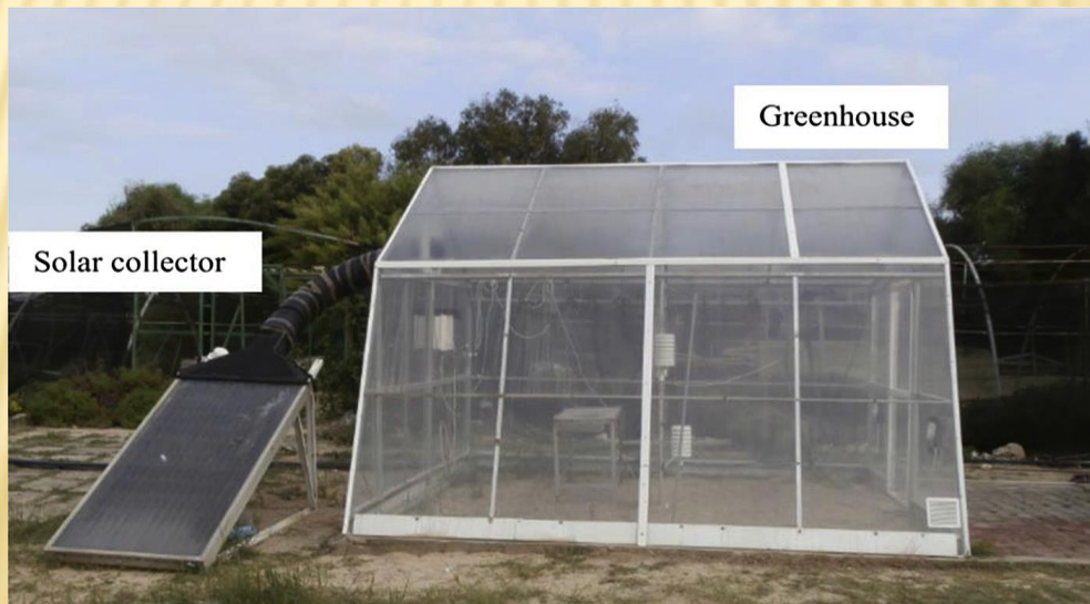
Greenhouse dryer attached with flat plate collector
