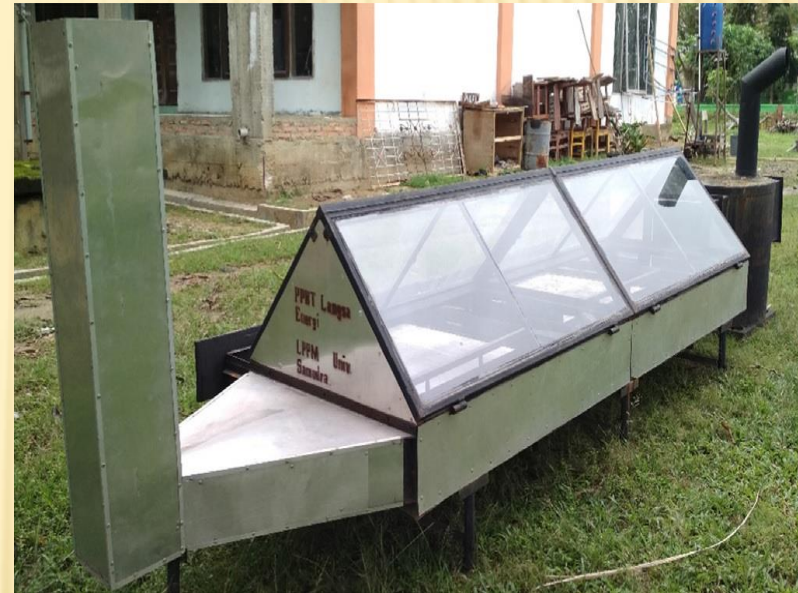
Setup of PVT mixed-mode dryer
