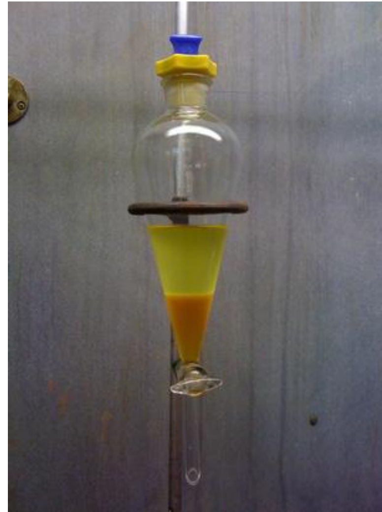
Figure 1: a) Schematic diagram of transesterification reaction b) Biodiesel separation layer
