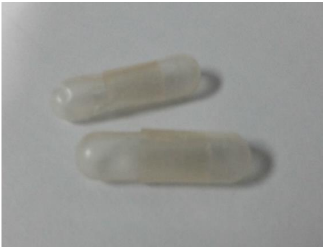
Photos of hard capsule samples through manual dipping process.
